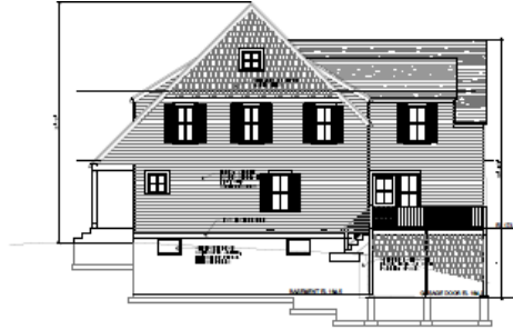
RIGHT ELEVATION (EAST) SCALE: 1/8" = 1'-0"
